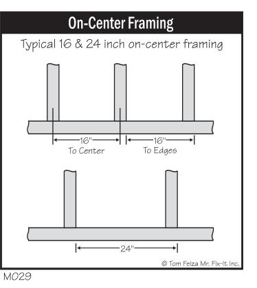
When the actual wall is assembled, allowances must be made for corners and for penetrations like window and doors, so not all stud spacing is 16 or 24 inch on center. For instance, windows are not always placed exactly between the standard 16-inch spacing, and you will always find additional studs and headers carrying the structural load around windows and doors. (Drawing S007)
